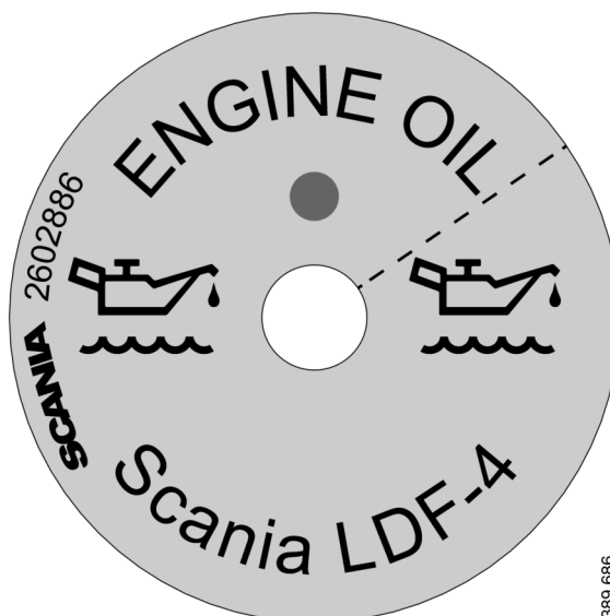
Oil filler label in the cylinder block.
